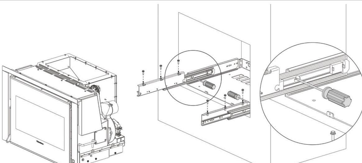
Block the rails with two screwdrivers and secure the flue pipe to the base with 6 screws.
