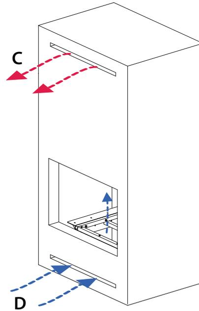
**C:** Air convection outlet. Minimum section 240cm<sup>2</sup>.
