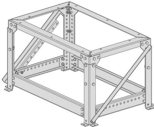
If there is no pre-existing chimney, one can be built using an insert-holder pedestal (optional kit). In fact, the latter fixes the insert to the ground.
