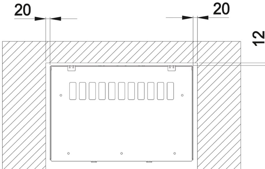
For the insert to operate correctly, a **minimum** side of 20 mm and rear space of 12 mm must be guaranteed; the coatings must be made of **non-flammable** material.
