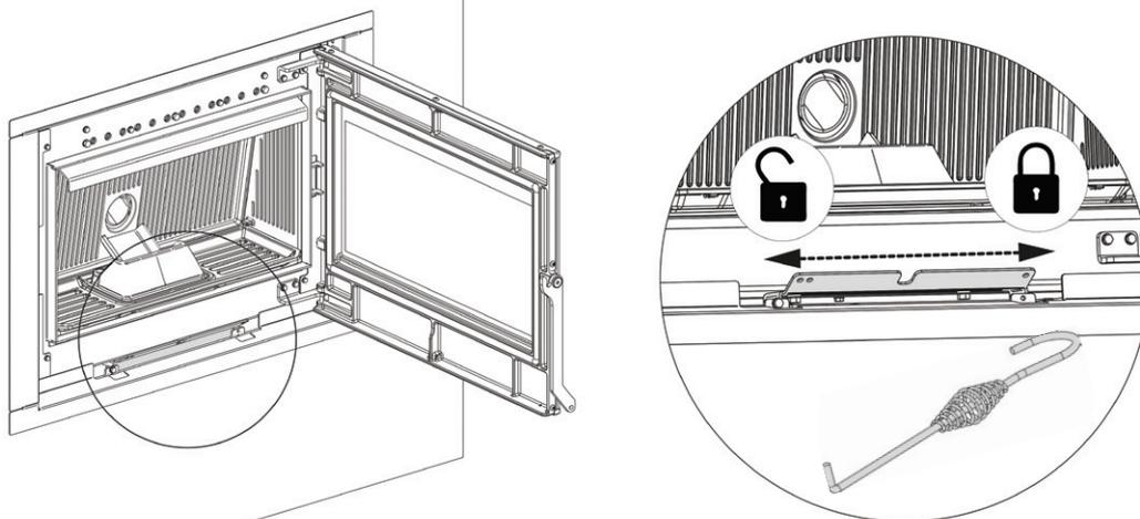
Close the insert and block the latch.
