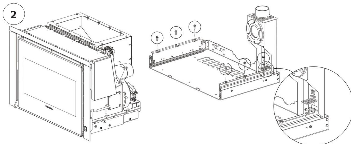
Remove the 6 screws and release the chimney from the bottom and install the feed bracket.
