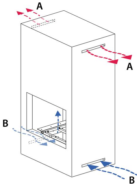
**A:** Air convection outlet. Minimum section 120cm<sup>2</sup>.
