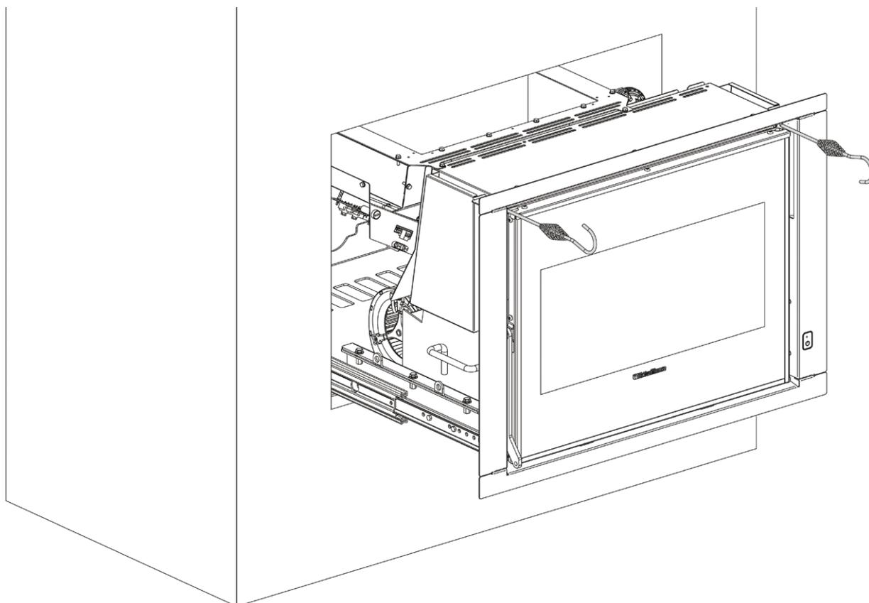
Use the holes on the two sides to remove the insert using pokers.
