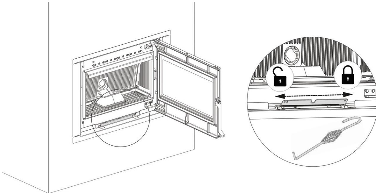
Use the poker supplied to perform the release/block operation.
