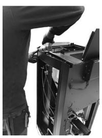
Fig. 52 - Remove the compensator
