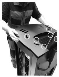
Fig. 51 - Remove the cover
