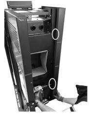
Fig. 59 - Secure the front side panel
