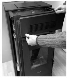
Fig. 28 - Remove the panel
