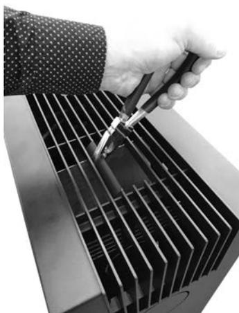
**Fig. 50 - Remove grid**
