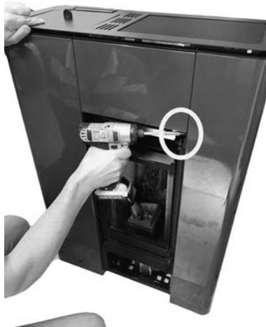
**Fig. 45 - Screw removal 2**
