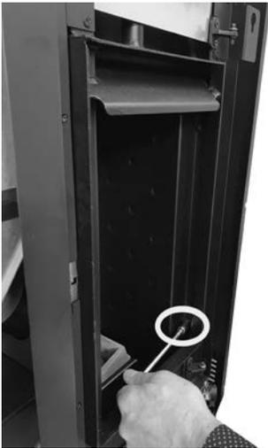
**Fig. 66 - Remove screw 1**
