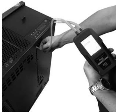
Fig. 62 - Connecting the digital pressure switch
