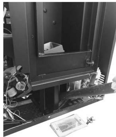
*Fig. 65 - Vacuum out the ash*
