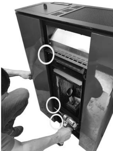
**Fig. 47 - Screw removal 3**
