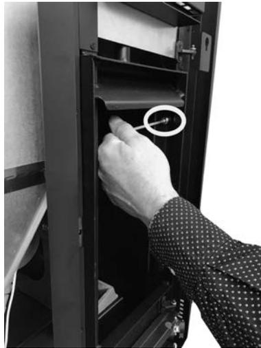
**Fig. 67 - Remove screw 2**
