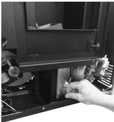
*Fig. 64 - Remove the inspection cap*
