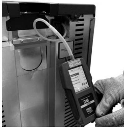
*Fig. 89 - Digital pressure switch connection (Atena<sup>3</sup> Plus12/14 - Duke 12/14 At - Saba 12/14)*
