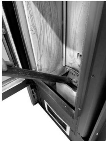
**Fig. 92 - Vacuum out the ash**
