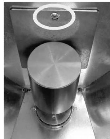
*Fig. 112 - Remove the screw*
