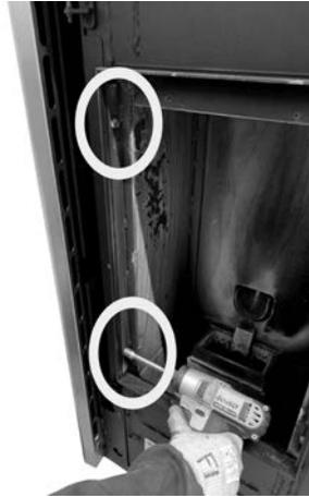
**Fig. 97 - Remove the hex screws**
