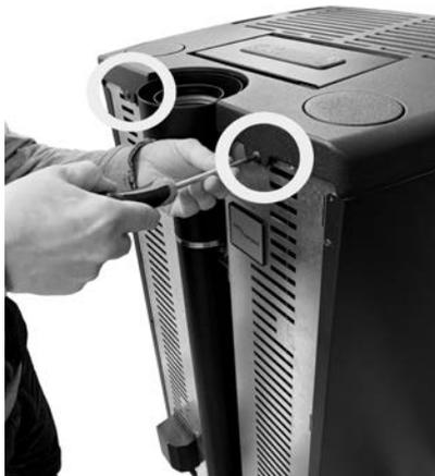
**Fig. 20 - Remove the screws**
