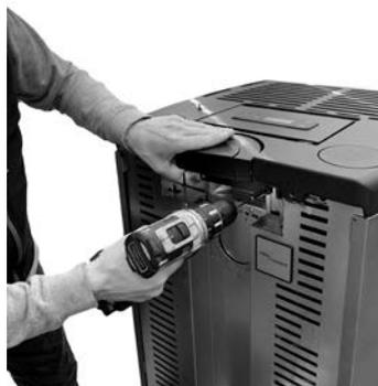
*Fig. 49 - Remove the cap (Atena<sup>3</sup> Plus 12/14 - Duke At)*
