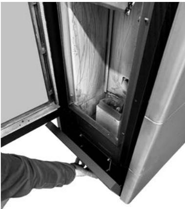
*Fig. 30 - Remove the front panels*
