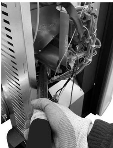
*Fig. 108 - Room fan cleaning (Atena<sup>3</sup> Plus 12/14 - Duke 12/14 At - Saba 12/14)*
