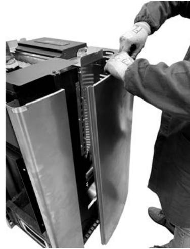
*Fig. 29 - Remove the side panels*
