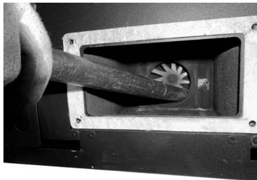
*Fig. 107 - Vacuum out the ash*
