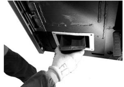
*Fig. 106 - Remove the fume diverter*
