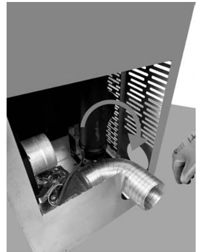
*Fig. 73 - Rotate the hose*
