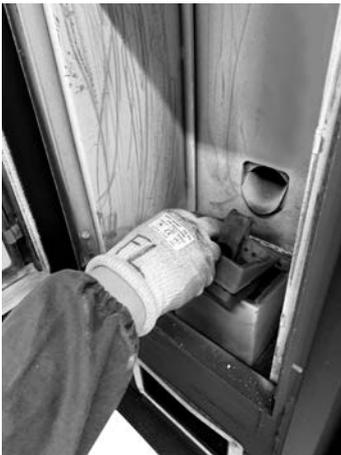
**Fig. 91 - Remove the burning pot**
