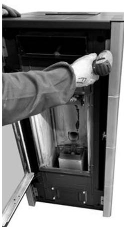
**Fig. 26 - Remove screws**
