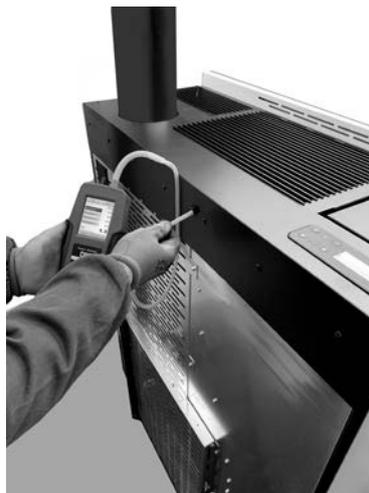
*Fig. 90 - Digital pressure switch connection (Mithos<sup>3</sup> Plus12/14)*
