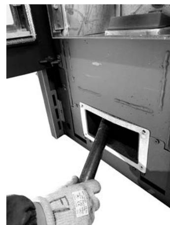
**Fig. 103 - Vacuum out the ash**
