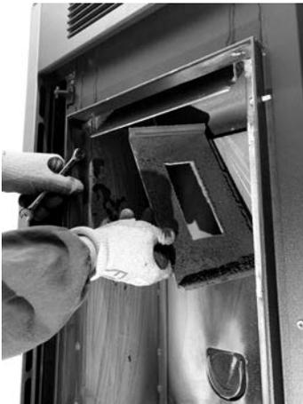
**Fig. 99 - Remove the head of the firebox 2**
