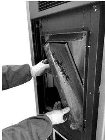
**Fig. 100 - Remove the side walls**
