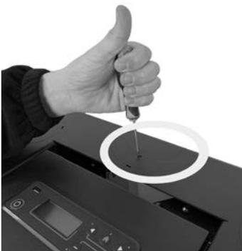
*Fig. 48 - Remove the cap (Saba 14)*
