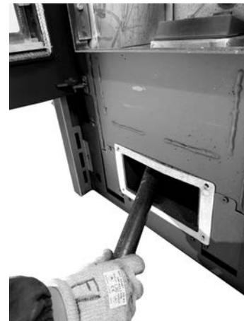
**Fig. 95 - Vacuum out the ash**
