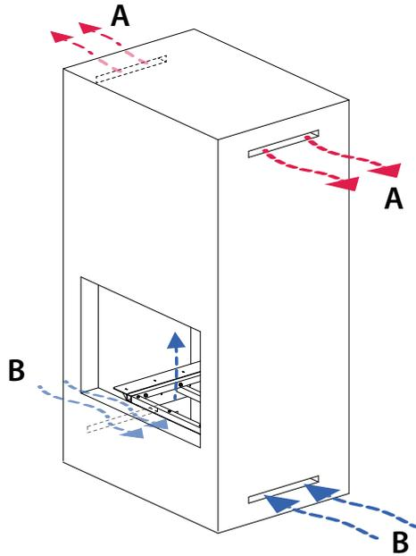
**A:** Air convection outlet. Minimum section 120cm<sup>2</sup>.
