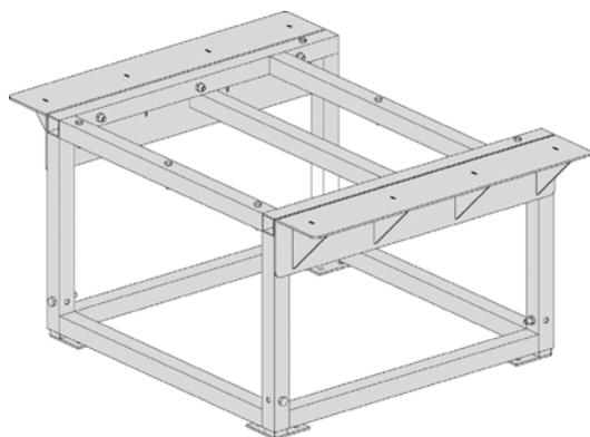
If there is no pre-existing chimney, one can be built using an insert-holder pedestal (optional kit). In fact, the latter fixes the insert to the ground.
