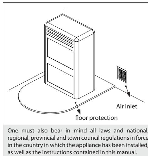
In the presence of type B gas appliances with intermittent operation not intended for heating, they must have their own aeration and/or ventilation opening.
