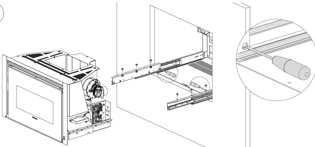
Block the rails with two screwdrivers and secure the flue pipe to the base with 6 screws.
