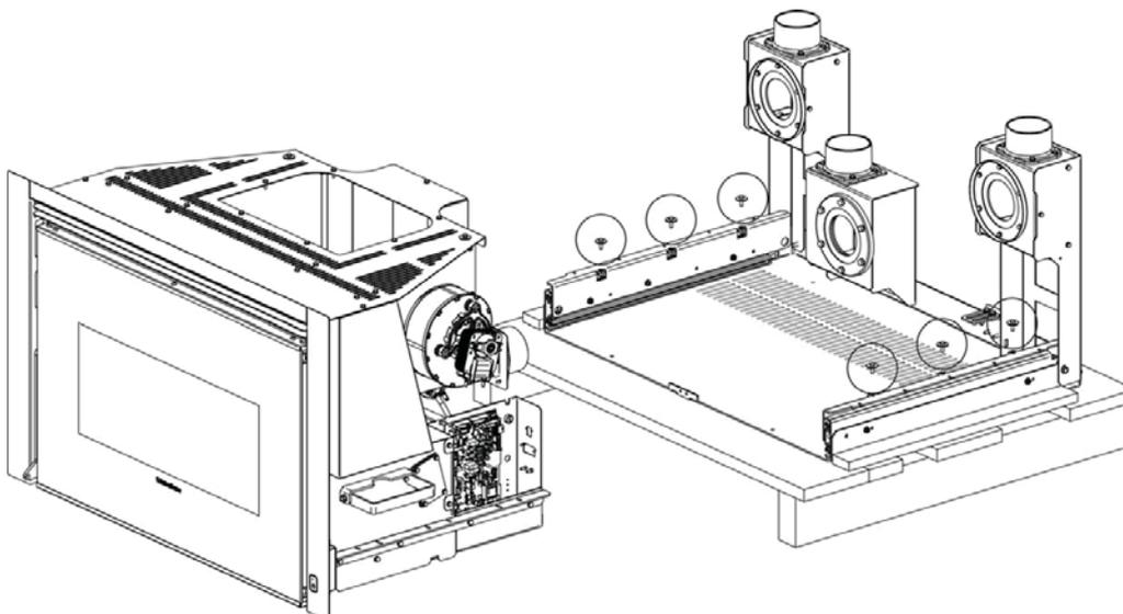
Remove the 6 screws and remove the flue pipe from the base.
