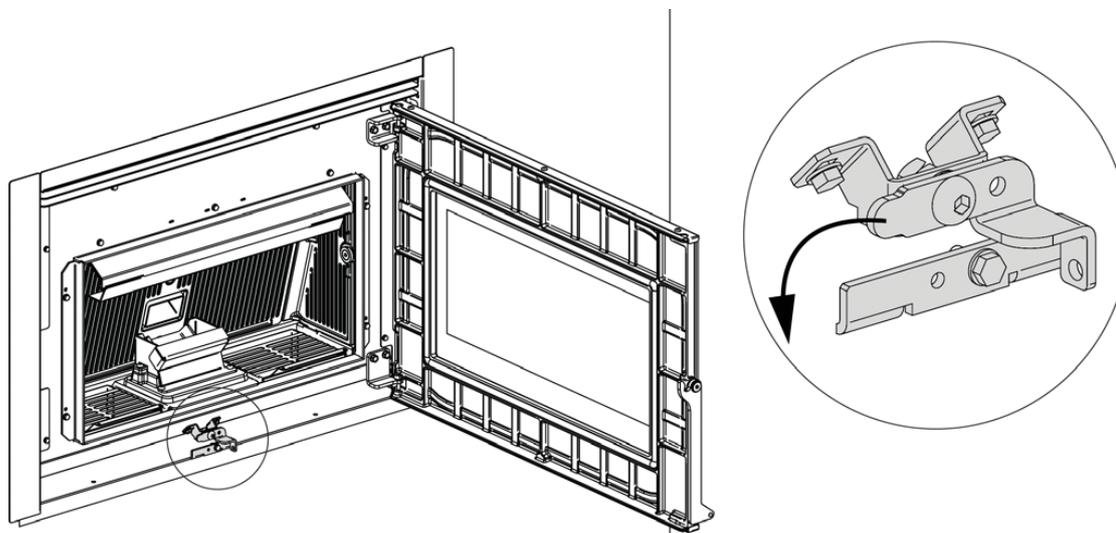
Close the insert and block the latch.
