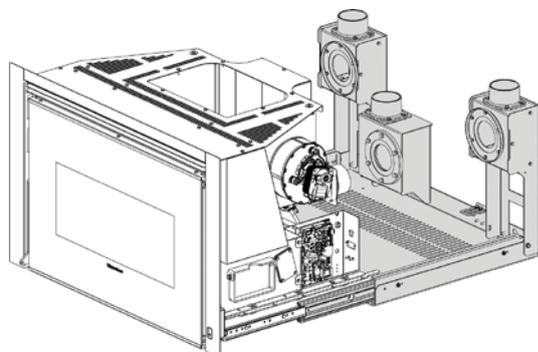
The insert is supplied with a sliding base in iron that allows it to be installed in a pre-existing chimney.
