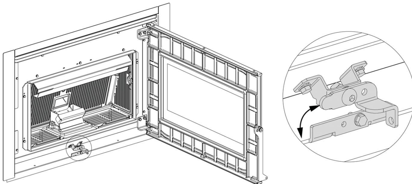
Use the poker supplied to perform the release/block operation.
