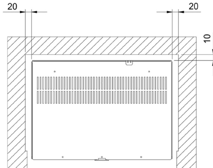
For the insert to operate correctly, a **minimum** side of 20 mm and rear space of 10 mm must be guaranteed; the coatings must be made of **non-flammable** material.
