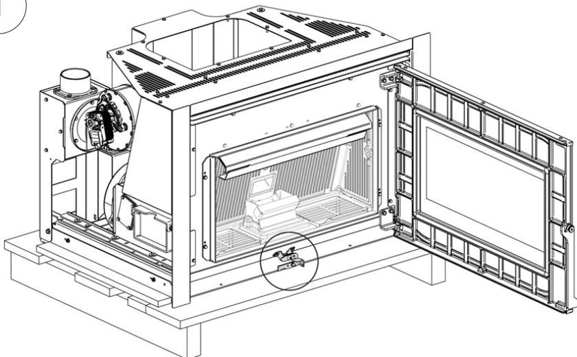
Open the door and release the latch using the poker supplied.
