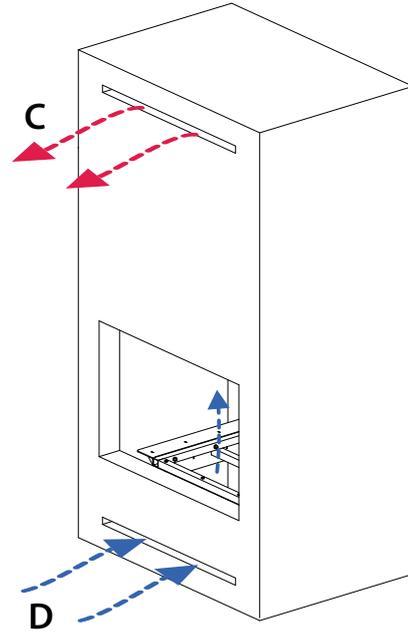
**C:** Air convection outlet. Minimum section 240cm<sup>2</sup>.
