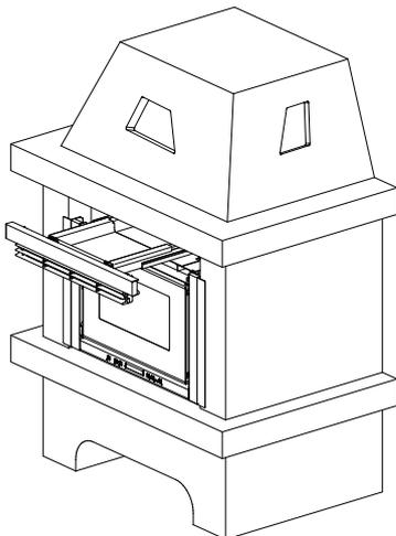
The optional pellet feeding kit allows pellets to be fed into the feed-box from the front without having to extract the insert (operation that requires machine switch-off).
