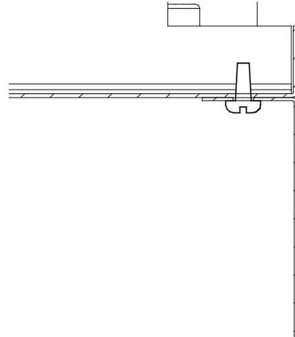
The 2 side frames are fixed to the upper frame by means of 2 screws each side.
