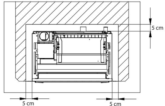
For correct functioning of the insert, during construction of the flue the measurements between the insert and internal walls of the flue must be respected (figure below).
